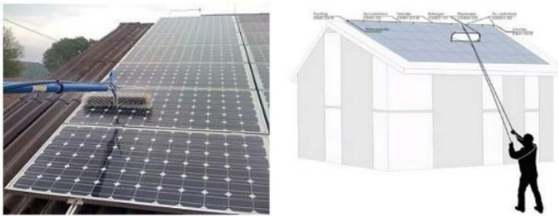
Fig. 2. Mechanical device for cleaning the rooftop SB
