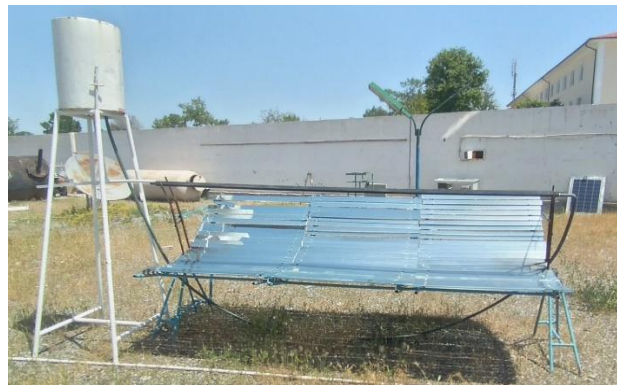
Figure 2.2. General view of the experimental parabolic trough solar collector.
