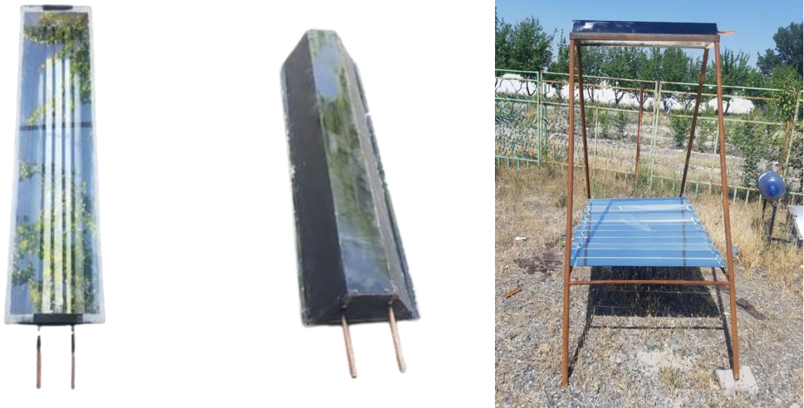
Fig. 1. Design, construction and evaluation of a Fresnel Linear Concentrator
