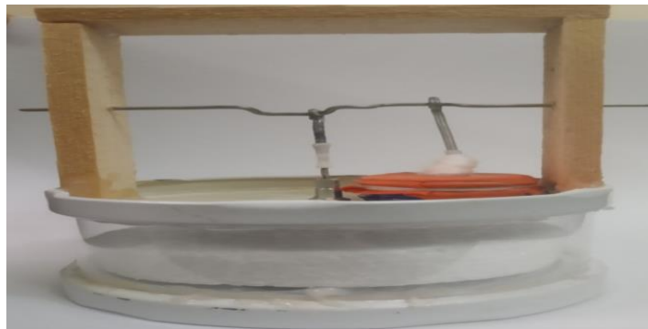
Figure 2. A practical Stirling engine operating at a low temperature difference.
