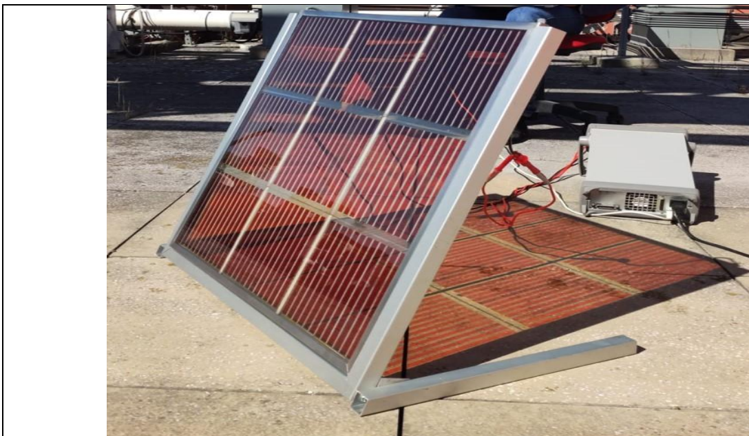
4-rasm. BIPV (Binoga integratsiya qilinadigan-Building-Integrated Photovoltaics) qo'llanmalariga mo'ljallangan yarim shaffof bo'yoqqa sezuvchan (dye-sensitized) quyosh moduli. University of Rome Tor Vergata
