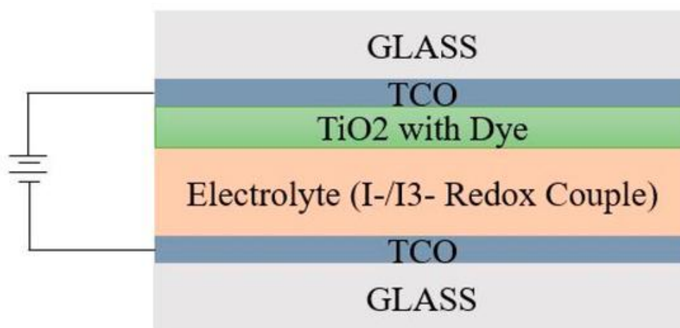
10-rasm. DSSC ning oddiy element arxitekturasini. ( https://doi.org/10.3390/en15228688 )
