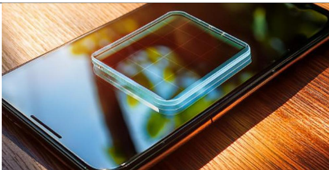
Figure 11: A small all-back-contact transparent solar cell (on top of a smartphone) developed by UNIST, South Korea. All the metallic electrodes are on the rear side, enabling a glass-like appearance. Such cells achieved ~15% efficiency with 20% visible transparency, and a module of them can directly charge electronic devices[65]. The image shows the clear solar cell module poised on a phone screen, illustrating potential integration into consumer electronics.
