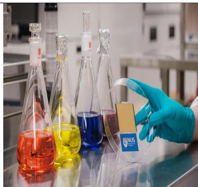
Figure 8b. The new perovskite-organic tandem cell (right) designed by NUS scientists can achieve a power conversion efficiency of 26.4%, outperforming the previous benchmark for similar devices.
