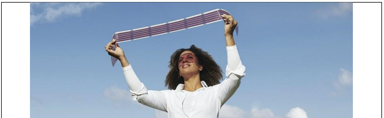
Figure 10: A researcher holds a flexible printed solar cell module. Thin-film solar cells (like organic or perovskite cells) can be fabricated on ultra-thin plastic foils using printable “solar inks.” These inks are deposited in layers onto flexible substrates via techniques such as micro-gravure coating, slot-die coating, and screen printing, producing lightweight, semi-transparent solar panels[19].
