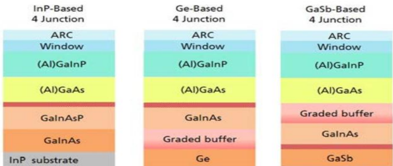
Figure 5. Different cell architectures for wafer-bonded 4-junctional solar cells. The bond is always indicated by the red line. Left: InP-based concept. Center: Ge-based concept. Right: GaSb-based concept. DOI: 10.1109/JPHOTOV.2017.2778567
