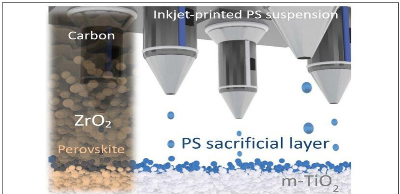
Figure 4: Conceptual illustration depicting an inkjet-printing process of sacrificial layer of polystyrene (PS) particles for nanoarchitecturing perovskite solar cell with carbonbased electrodes with solar cell structure depicted on the left(DOI: 10.48550/arXiv.2211.09424 ).
