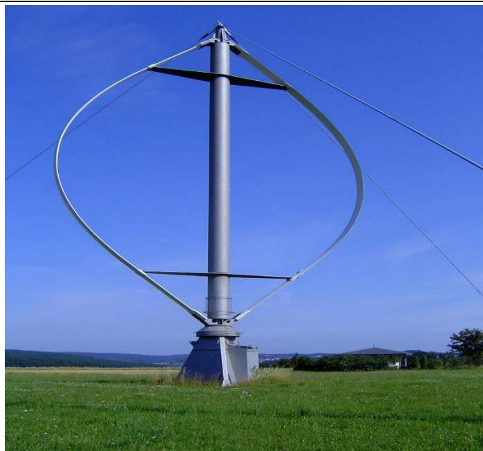
Figure 28. VAWT – Vertical Axis Wind Turbines. This is an image of a Darrieus wind turbine.
