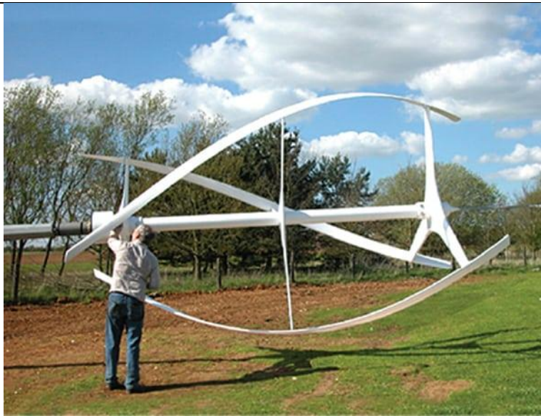
Figure 19. The quietrevolution. London-based quietrevolution's qr5 VAWT is designed to eliminate noise and vibration.
