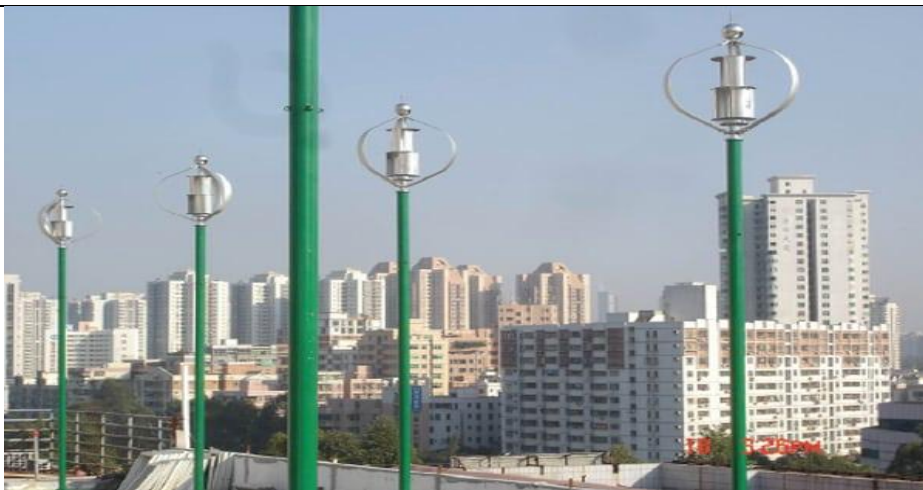
Figure 16 Maglev. When Chinese developers unveiled the magnetic levitation wind turbine at the 2006 Wind Power Asia Exhibition, it was hailed as a breakthrough in the evolution of wind technology. The technology is today used to power streetlights in Shenzhen and is available in ranges from 300 W to 1 kW.
