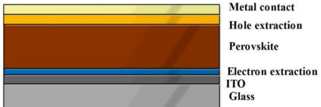
Figure 13. A schematic diagram represents the simple Perovskite Architecture.
