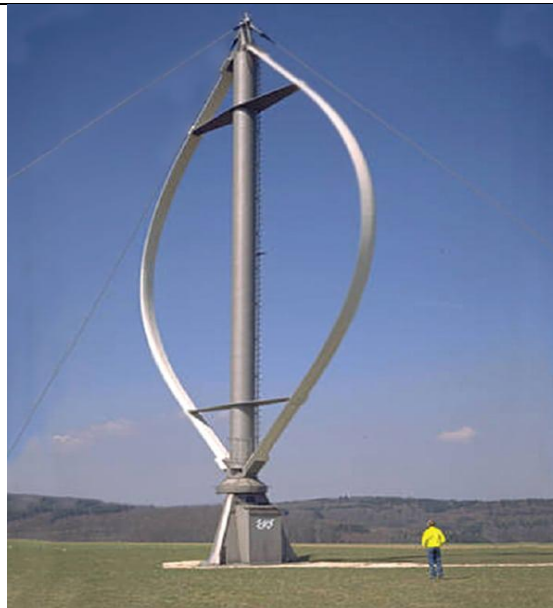
Figure 13. The Darrieus. French engineer Georges Darrieus' 1931 vertical-axis wind turbine design—shaped like an eggbeater—has resurfaced in modern times.
