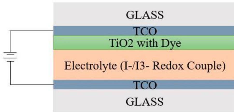
Figure 10. Simple cell architecture of DSSC. ( https://doi.org/10.3390/en15228688 )
