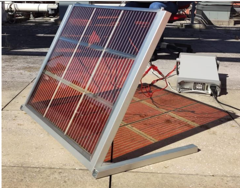
Figure 4 Semitransparent dye-sensitized solar module for BIPV applications University of Rome Tor Vergata
