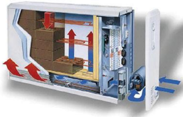
Figure-5.5.6. Storage heater section.
