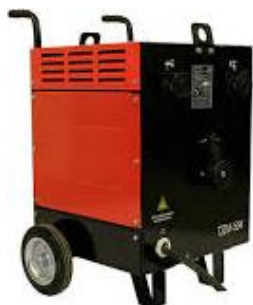
58-rasm. Payvatlash transformatorining tashqi ko'rinishi.
