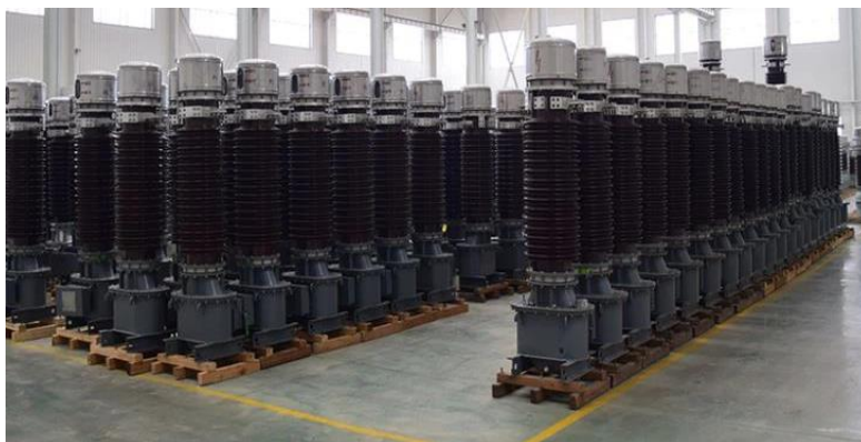
57-rasm. Kuchlanish transformatorining tashqi ko'rinishi.
