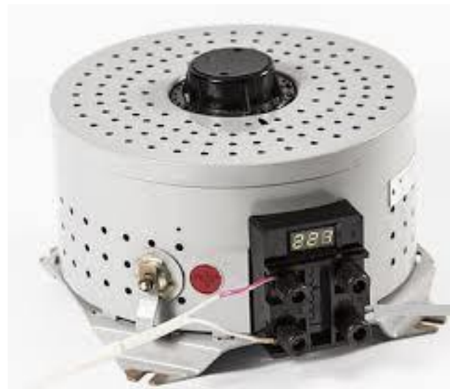
Figure 55. General view of a laboratory autotransformer.
