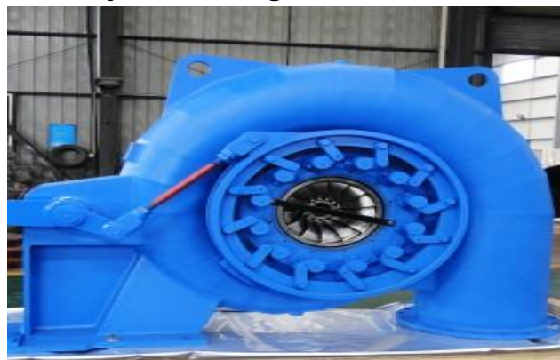
Figure 23. General view of a Francis hydroturbine.
