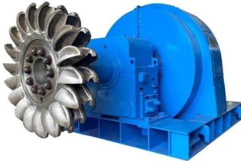
Figure 22. General view of a Pelton hydroturbine.
