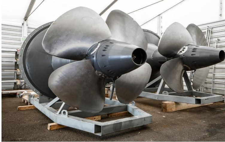
Figure 24. General view of a Kaplan hydroturbine.
