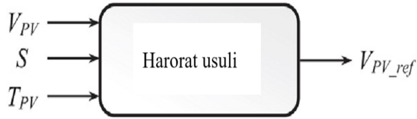
Fig. 2.15 Temperature method block diagram.
