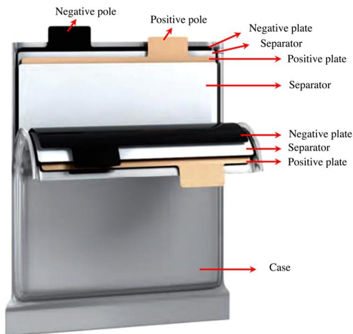
Fig, 5.15. Parts and general appearance of lithium-ion polymer battery.
