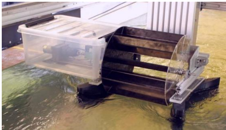
Fig. 6.3. Free-flow micro-HPP developed by Olivier Cleynen, Emeel Kerikous, and Stefan Hoerner.
