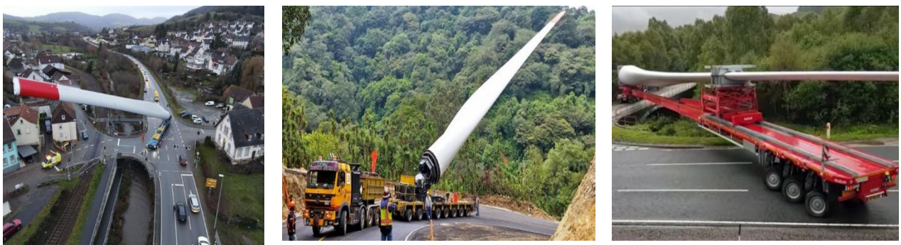
Figure 5.17. Transportation of wind turbine blades.
