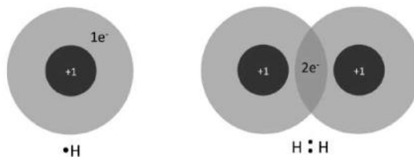
Fig. 1.10. The simplest form of covalent bonding between a pair of H atoms to form a H_2 molecule.
