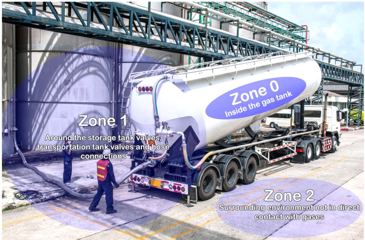
Figure 56: Illustration of zones (according to ATEX)
